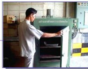
DEMOISTURIZING SPECIMENS BY USING OVEN
